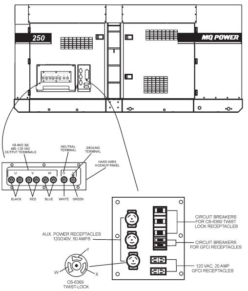
Figure 6. Output Terminal Panel
